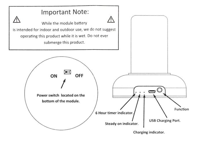
Note: This module can be used with a remote on and off device that is sold separately.
